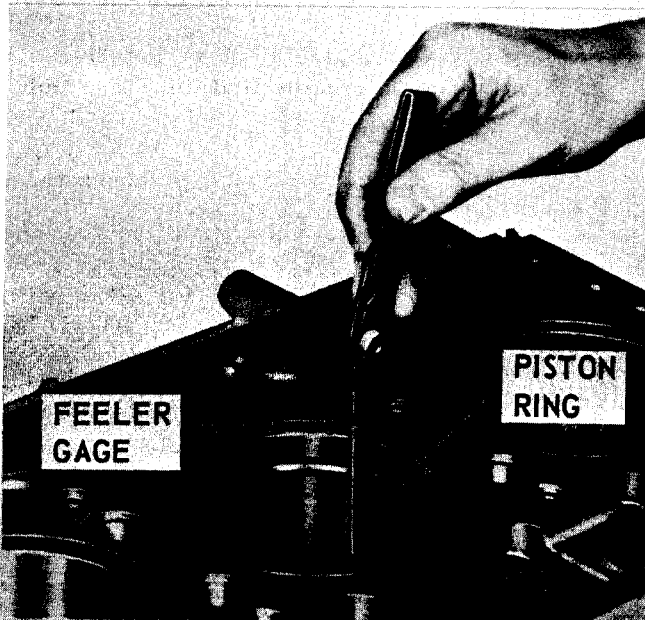
C MEASURING PISTON RING GAP
