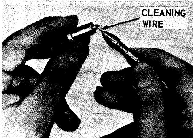
F CLEANING SPRAY TIP ORIFICES
