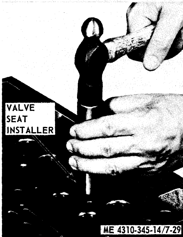
B INSTALLING VALVE SEAT INSERT
