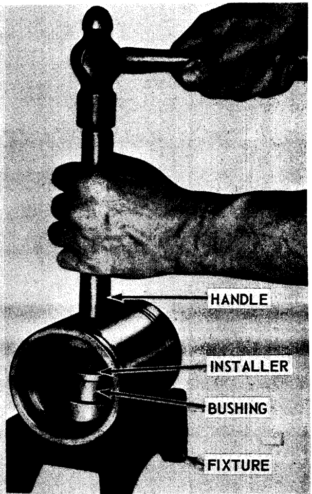
B REMOVING OR INSTALLING PISTON PIN BUSHINGS
