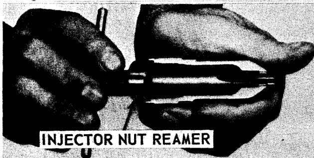
G CLEANING INJECTOR NUT SPRAY TIP SEAT
