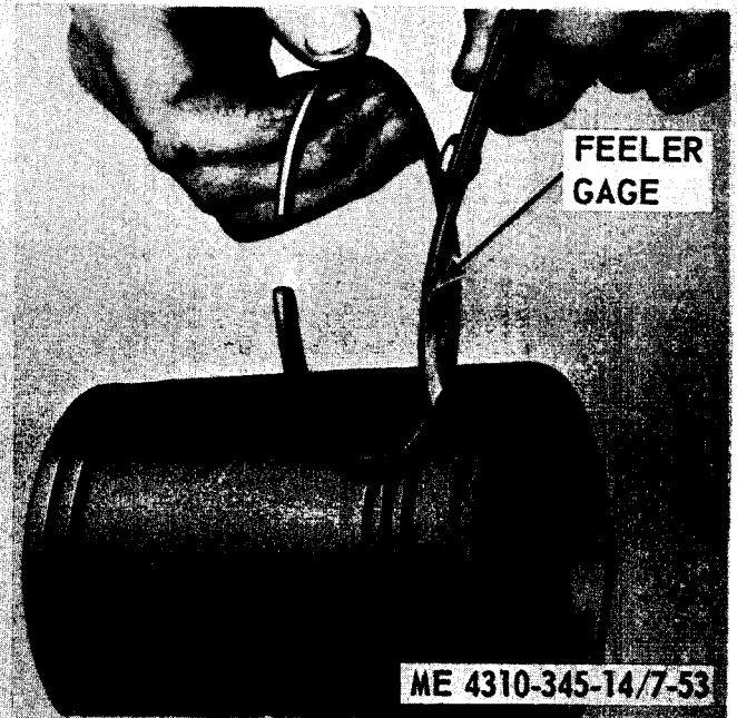
D MEASURING PISTON RING SIDE CLEARANCE
